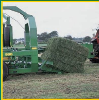
Conveyor loading of double bale
