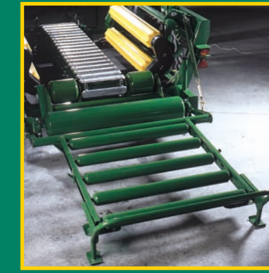
998 Unloading Conveyor Down
