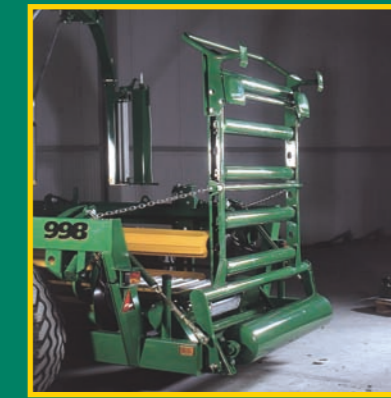
998 Unloading Conveyor Up
