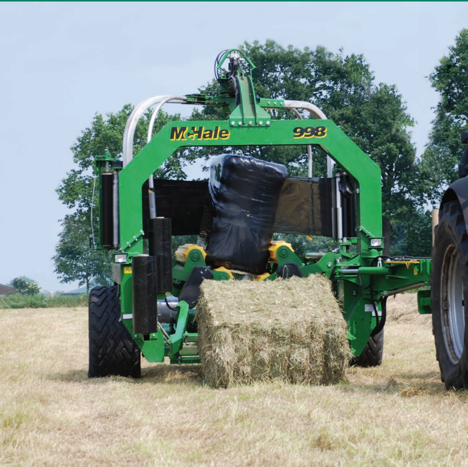
Conveyor loading of double bale
