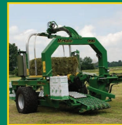
Lifting Bale to Wrapping Position
