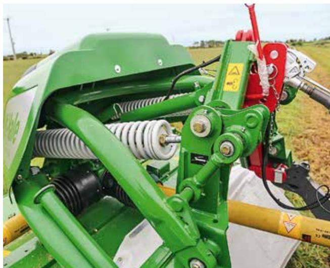
The mechanical double-ended link between the spring and frame maintains a more consistent tension as the mower works through its 500mm of suspension travel.
