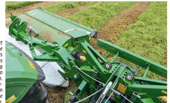
Bed pressure is set hydraulically on the dials; 100 bar is the norm. Ropes release the folding rams from field to transport position. Mechanical break-back can be seen at the front of the mower arm.
