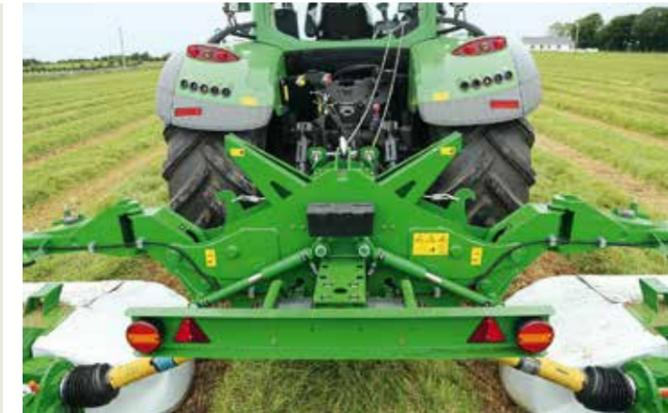
The amount of overlap is fixed at 150mm per side. Angled rams at the back provide the bed pressure, and each contains a 2-litre accumulator.
