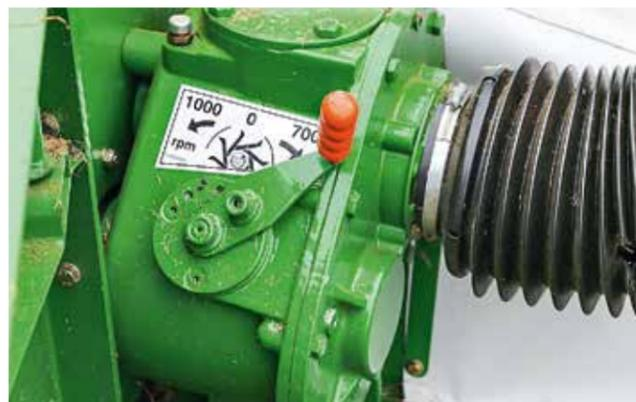
Conditioner speed is selected on the gearbox – 700 or 1,000rpm.
