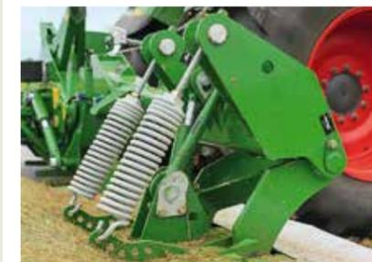
Coil springs maintain the cutterbar angle and, together with the mechanical link, allow the mower to lift up and back if it encounters an obstacle. The ram within the mechanism is linked to the raise/lower circuit and locks the bed against the stops when raised.
