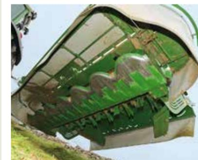
The seven-disc bed has been set to McHale spec and comes with full width stone guards.
