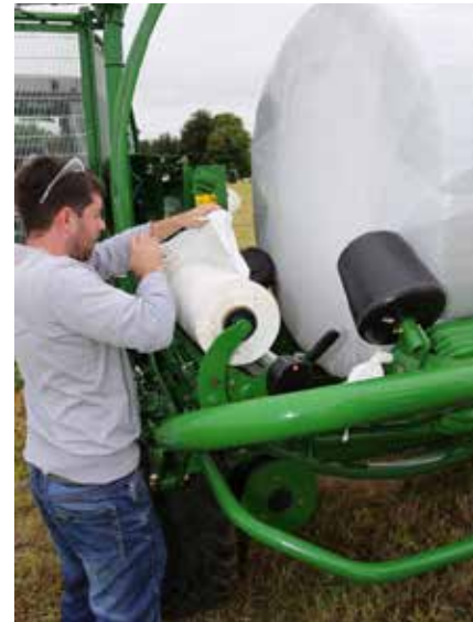
The rear gate swings open for loading new rolls of wrap. A safety switch stops the arms from moving with the guard open.
