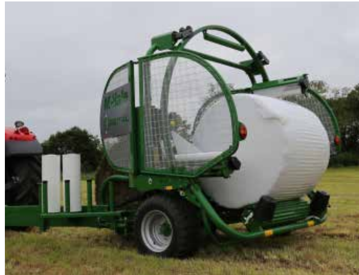
Just like the Fusion the rear roller swings down to lower the bale to the ground. The rear roller position can also be adjusted to cater for bales up to 1.48m in diameter.
