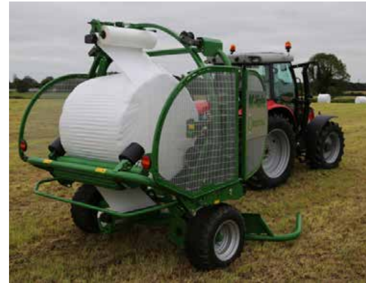
The twin film dispensers can spin at up to 40rpm, a significant increase on the HS2000 wrapper's 26-28rpm.
