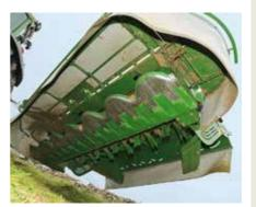
The seven-disc bed has been set to McHale spec and comes with full width stone quards.
