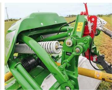
The mechanical double-ended link between the spring and frame maintains a more consistent tension as the mower works through its 500mm
