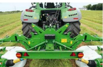
The amount of overlap is fixed at 150mm per side. Angled rams at the back provide the bed pressure. and each contains a 2-litre accumulator.
