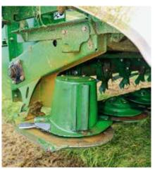
500mm of travel. It's a clever and simple system that worked effectively during our time with the mower. In fact the whole combination performed well and produced a neat square-edged row for easier handling by whatever machine follows on behind. The front mower is raised and lowered by its own hydraulic ram. In testing this ram delivers 650mm of ground clearance when the mower is raised at the headland.
