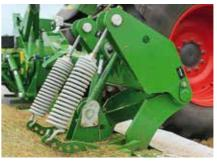
Coil springs maintain the cutterbar angle and, together with the mechanical link, allow the mower to lift up and back if it encounters an obstacle. The ram within the mechanism is linked to the raise/lower circuit and locks the bed against the stops when raised.
