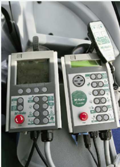
On the Fusion 2 model, the RDS Expert Plus control box (left) replaced the RDS Expert. The latter has a separate raise/lower control for the baler's pick-up.
