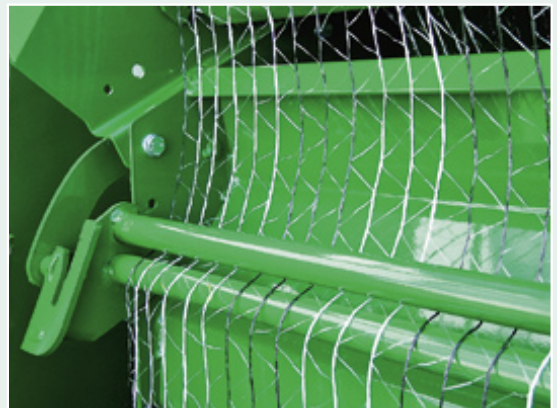
Net wrap feed on the original Fusion baler wrapper passes through a single bar tensioner. Easy to thread and reliable, the critical check is to ensure the rubbing surface is kept smooth and shiny for the best possible performance.
