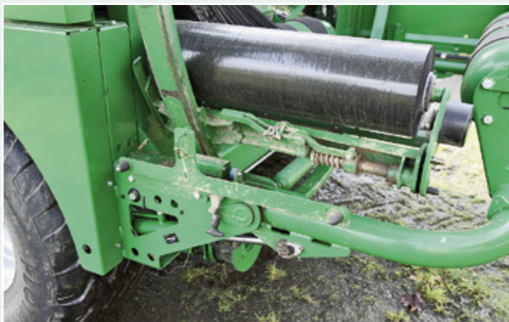
Detail changes have been made to various areas of the Fusion, including the latest Fusion 2 featuring a spring return on its film roll retention latch. The wrapper ring should lock when the rear cover is opened.
