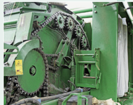
The Fusion 2 has a double-bar net tension system for a tighter wrap. This is useful when baling hay and straw.
