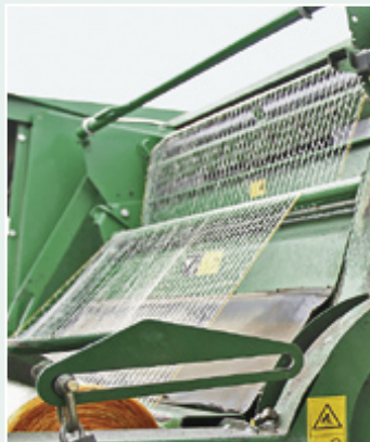
Net wrap feed on the original Fusion baler wrapper passes through a single bar tensioner. Easy to thread and reliable, the critical check is to ensure the rubbing surface is kept smooth and shiny for the best possible performance.
