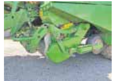
Pick-up reel: The pick-up reel is an essential part of the machine and must be maintained to a very high standard.
