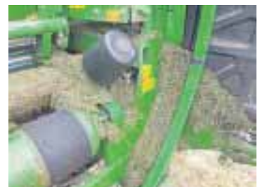
Cleaning: This build-up of grass around the wheel arches should be cleaned down daily.
