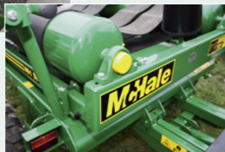
... with models from 1992 having their brackets moved out to 'deepen' the well retaining the bale. Note subtle change to chassis design.
