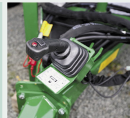
The 991BJS uses the current servo-hydraulic joystick control, and benefits from increased automation that includes auto tip and load. Electronic control has been available since 1995 on the BE, which is, today, the most popular model.
