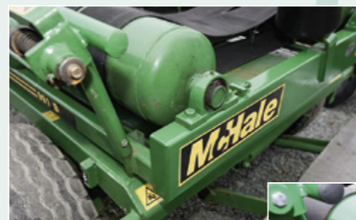
Original 991 belt roller brackets mount some way from the edge of the table frame...
