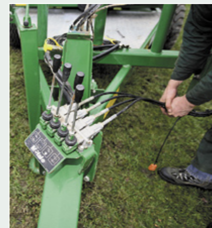
Later version of cable control. A detent allows the bale rotation lever to lock back to complete the wrapping cycle automatically, but load, tip and cut remain manual. Most 991B wrappers have been converted to 991BC 'cable' spec, conversion kits costing £350.
