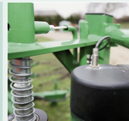
Film break sensor comes as part of the BE electronic control package, the 991BE wrapper now outselling all other variants. Film dispenser post and roll release design changed to still current design in 1998. All electronic models can be operated via remote control, a kit costing around £350. BE remains a rare used find.
