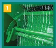
After the bale full alarm sounds on the control box, the net tension bars pivot forward allowing the net to feed into the bale chamber unrestricted.
