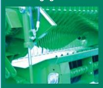
This widens the feed channel and on re-engaging the PTO the blockage can be fed through.
