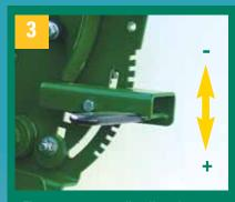
The operator can easily adjust the amount of net being applied by simply moving the adjustment handle on the netter.
