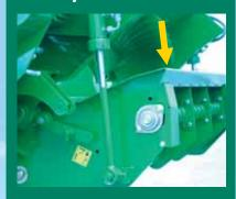
Should a blockage occur the sound of the slip clutch alerts the operator who can hydraulically lower the floor from the tractor cab.
