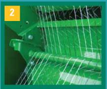
As the net comes into contact with the bale the net tension bars pivot back, applying maximum pressure. This ensures efficient net usage and that a tight layer of net is applied to the bale.
