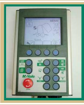
The F560 is controlled with an Expert Plus Control Console, which features a large graphic display, this allows the operator to monitor the baling process graphically from the control console. It also features;
