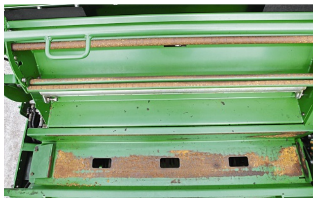
Blanks (green, below) should be installed whenever knives are removed. Original blades are slightly shorter than the post-2008 current design (black), which is now the standard replacement for all models. Balers have 15 blades but are often used with fewer.
