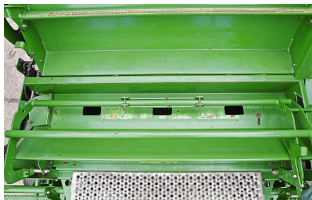
Original net wrap box adjusts from one end and has a single-arm net guide (left), whereas later 2008 balers (below) gain two adjusters in the box and a twin-arm net guide. On all machines, ensure net guides are cleaned of any rust before starting work.
