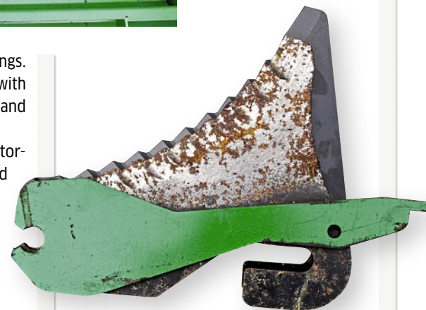
Blanks (green, below) should be installed whenever knives are removed. Original blades are slightly shorter than the post-2008 current design (black), which is now the standard replacement for all models. Balers have 15 blades but are often used with fewer.
