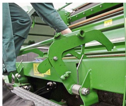
Net knife pivot needs to allow the unit to drop with a distinct bang. As with all elements of the net wrap system, check the pivot points are free. Serrated knife cuts the net in the 'V'. If blunt, the net is inclined to tear. The knife is easy to renew.
