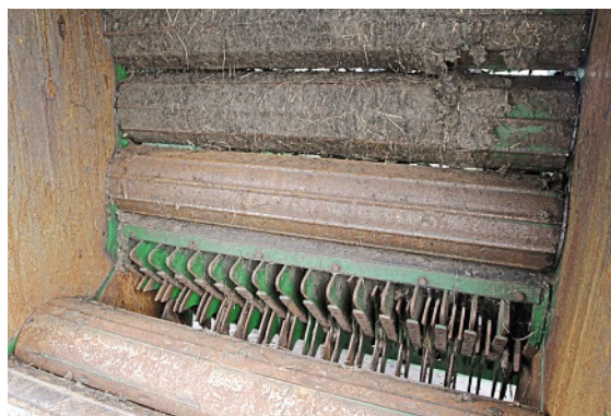
Debris can accumulate on lower rollers on early models (far left), although a scraper prevents this build-up on 2008 models (left). If not cleaned off for the new season, the bottom roll can break the net on the first few bales.
