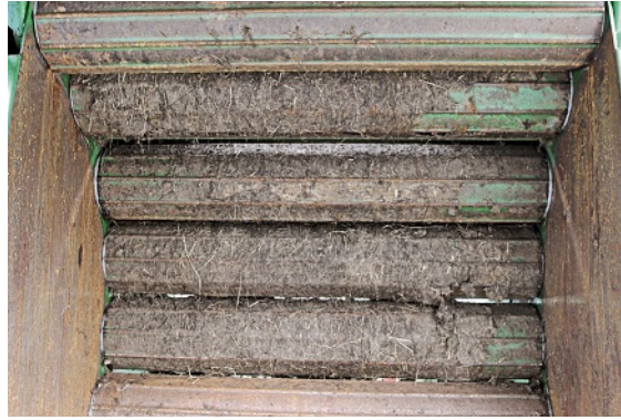
It's easy to spot the blanking plate in original F550 balers (far left); later 18-roller models perform better in dry, brittle straw. Where rollers are dirty, inspect underneath for wear and damage.
