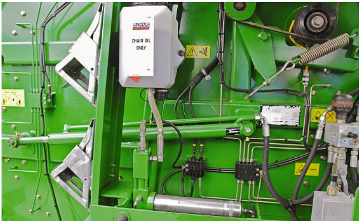
Original auto-lube grease and chain oiler system (left) works every time the rear door opens. In contrast, post-2008 greaser (below) operates in the same way, but the chain oiler (below, inset) moves to the nearside of the baler and has full-time drive from the end of the feed rotor.
