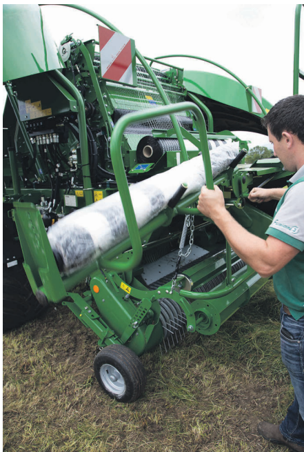
This cradle makes it easier to load rolls of net onto the platform.
