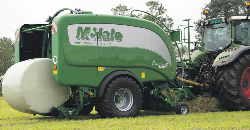
The Fusion 3 Pro has an optional bale weighing system utilising the wrapper table. This and other information such as bale moisture and job count can be printed off for each customer.
