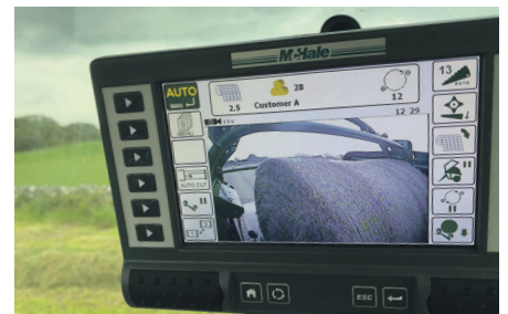
The Itouch display automatically flicks from the main information screen to a camera feed showing the bale transfer and drop off. ISOBus is an option on the Pro and Plus.
