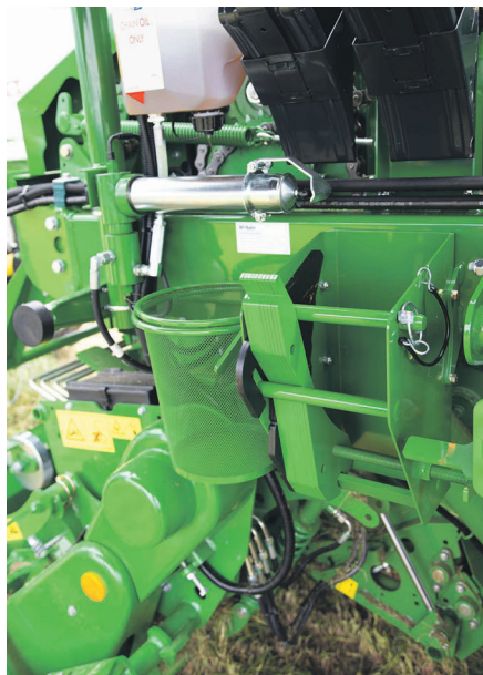
A storage bin has been added under the greaser for new and old cartridges.
