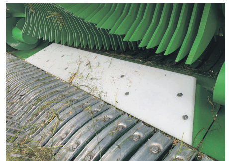
To enhance crop flow this nylon plate has been added, it tightens the gap between the rotor and intake. The plate can also move down slightly as a first line of defence to dealing with lumps or larger rows.
