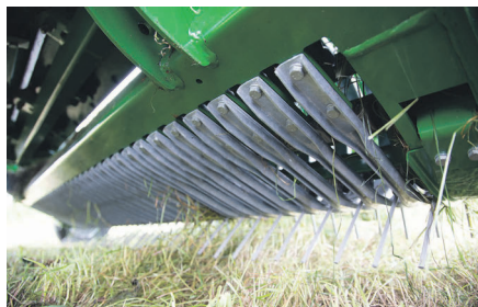
The bands narrow underneath, allowing any broken tines to fall out rather than remaining rattling around and taking out its neighbours.
