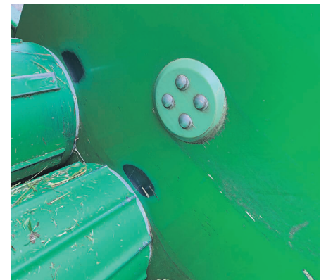
The moisture sensor is positioned in the side of the bale chamber.
