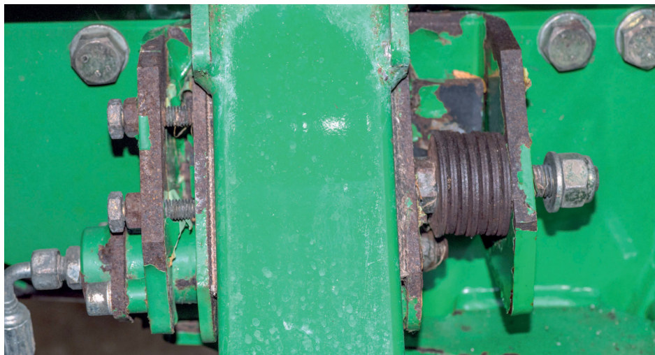
Ring Holding Device secures the wrapping ring to ensure it is correctly positioned ahead of wrapping the next bale. If you can't see any friction material, new pads will be needed.
