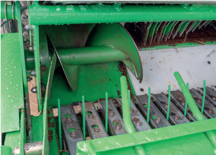
A key development in 2016 was the switch to larger diameter side augers, the rotor also growing in diameter. The floor under the rotor was also changed from solid to suspended to smoothen crop flow; balers from 2018 (right) have the flex nylon pad also mounted on rubber blocks.
