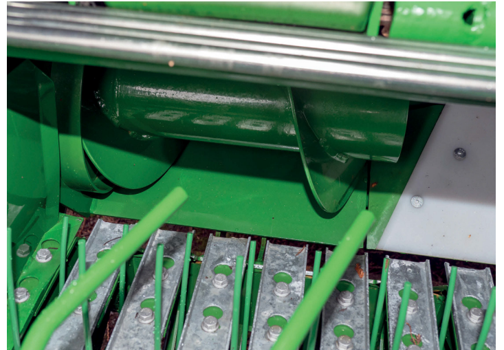
A key development in 2016 was the switch to larger diameter side augers, the rotor also growing in diameter. The floor under the rotor was also changed from solid to suspended to smoothen crop flow; balers from 2018 (right) have the flex nylon pad also mounted on rubber blocks.
