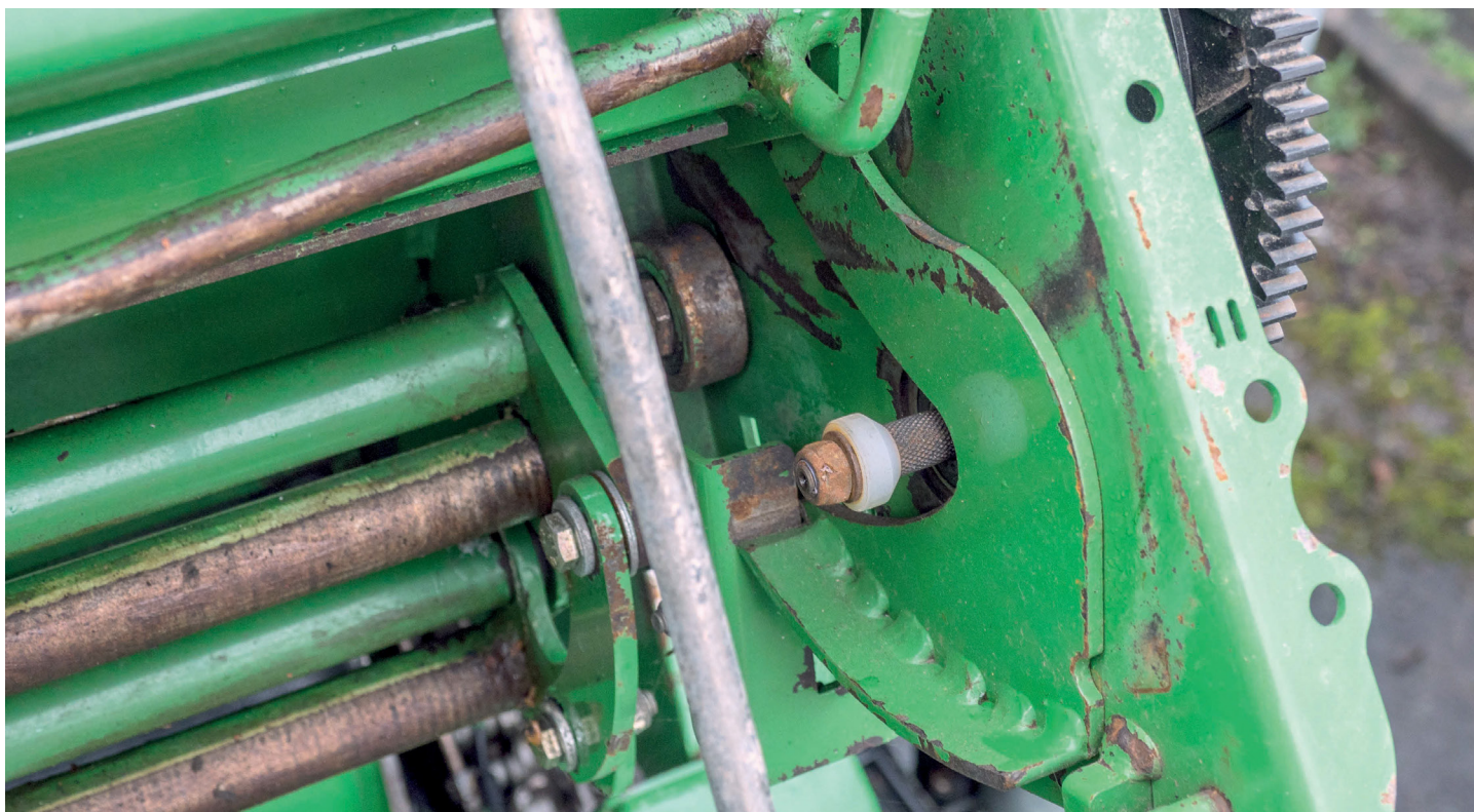
The net wrap cut system is simple and robust but, over time, the nut that releases the net hook wears and will need renewing.
