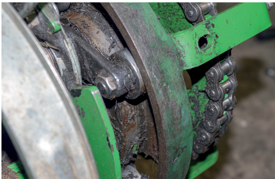
Play in the tine carriers? The cam bearings may need renewing (above), and the cam track itself should be replaced if you feel a wear lip. The track material was made from cut steel originally, changing to cast and now to a cast and hardened design. The latter can last for 40,000 bales plus.
