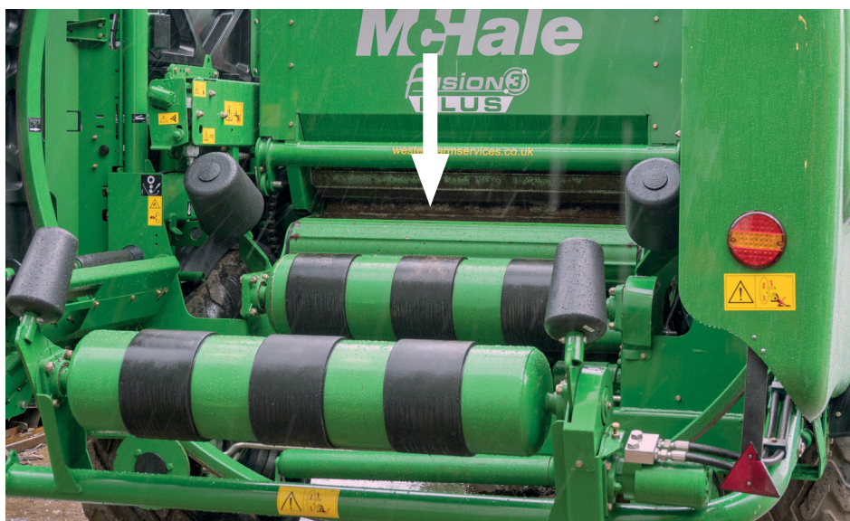
The solid bar ahead of the wrapping table (arrowed, above) was replaced by a roller (arrowed below) from 2016. This smoothens chamber-to-wrapper bale transfer, although the earlier design still works reliably.
