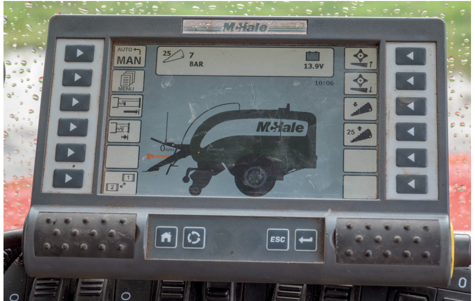
Fitted as standard to the Fusion 3 Plus, the McHale iTouch controller displays live images from two cameras as standard. Split camera and menu screen came as a part of the package from 2017.
