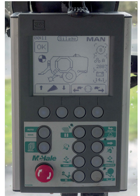
Expert Plus Control Console is standard on the Fusion 3. A lube check alarm for both grease and oil levels is included, so there is no excuse for dry chains and oil-starved roller bearings. A selectable knife option allows the knife sets to be changed from the tractor cab.
