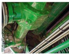
The main bevel gearbox is a simple unit, with power divided to drive the pick-up and rotor on one side, the bale chamber on the other. The oil in the box should have been changed at the first service and then at least once a year. Look for leaks at the input shaft seal and check for play. Note easy access to drain plug.
