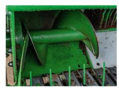
The side augers on the original V660 balers have a slimmer central core, with the very first models having a steel as opposed to white polymer drop floor as pictured. Check for play in the auger bearings.
