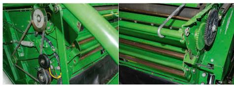
Up until 2018, V660 and other models in the McHale range used the established mechanical net wrap system with belt driven roller and bar guides. The bars benefit from a light going over with emery cloth if they are rusted, with any nicks in the bars needing to be removed to avoid net snag. The net wrap cut system is simple and robust but, over time, the nut that releases the net hook wears and will need renewing.
