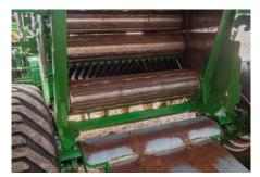
Incoming material is fed into the chamber via a pair of fixed rollers, with a third upper roller helping to shape the material as the belts expand to accommodate the growing bale. The lower roller bearings work hard, so ensure they are in good order, particularly on a baler with a high bale count.
