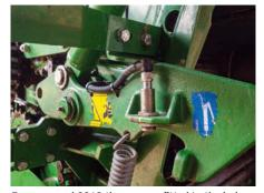
From around 2012 the sensors fitted to the baler were changed to a design that unscrews from the wiring harness, making swapping out a failed item easier and less costly. All the sensors are of the same type. Both tailgate locks have a sensor on later V640/V660 and V6740/V6750.
