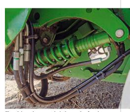
The pick-up is suspended via a pair of springloaded hydraulic cylinders. The pick-up wheels provide anti-scalp protection as opposed to support in work. Take a good look at this area of the baler as operator abuse can lead to damage to include broken springs. Also look for leaks in the pressurised oil lines, typically caused by something, such as a large stone, catching under the pick-up.
