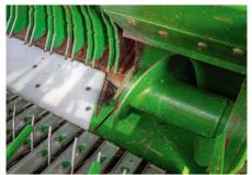
In 2019, the last year of V640/V660 baler production, McHale changed to a revised side auger design with a fatter centre shaft with the end angled to improve crop flow. This design is carried over to the current V6740 and V6750 models
