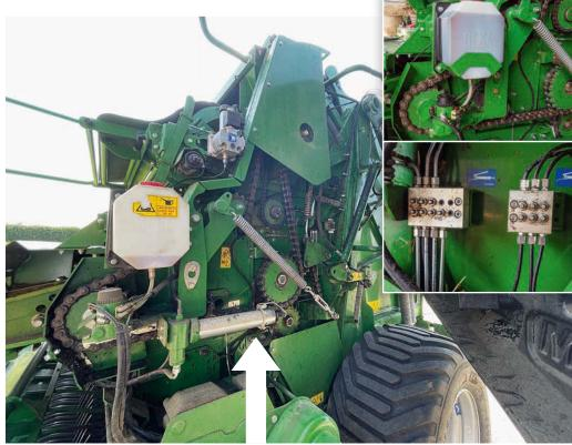
A continuous oiling system is used on all V640 / V6740 and V660 / V6750 balers. All models have centralised grease points (inset lower) with an automated system as an option (arrowed). The oil tank (inset upper) needs a top up every 300 bales.
