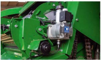
From 2019, McHale switched to a new hydraulic net brake system, this enabling net to be fed into the bale chamber more easily at the start of wrapping with the system progressively applying a braking force. It can be adjusted from the tractor cab to suit different qualities of net, to include allowing greater tension to be applied to a high tensile net. This in tun can be exploited to reduce the length of net consumed to wrap the bale.
