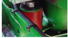
A pair of easily checked 'rubber' blocks provide a cushion for the drop floor, enabling clumps of crop to pass under the feed / chopping rotor with a reduced chance of blockage. If the intake does block, the drop floor can be lowered from the tractor cab to allow it to clear.
