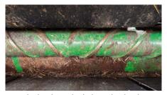
In work, the pictured spirals on the cleaning auger roller will clear debris from the belt rollers. Debris collects in the area, balers stored wet possibly suffering corrosion on the rolls that will typically be worn off in work. The double drive system fitted to V660 and V6750 chopper balers includes an extra belt drive roller above the pictured plain roll, this helping ensure the belt does not slip when rolling a heavy bale of chopped material.
