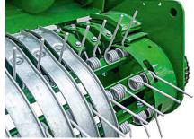
A six tine-bar camless pick-up was first offered as an option on V660 balers from around 2016 and is an increasingly popular choice on current V series balers. Well suited to faster working speeds and heavy crops, the design is maintenance free. The pick-up is the same 2.10m working width. Tines work hard and stripper bands can get damaged, so inspect carefully.
