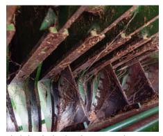
The knives in the chopping rotor can be sharpened with an angle grinder, but this needs to be done carefully to avoid taking away too much metal or overheating the metal. If possible, check the blades against a new one. Blunt knives obviously consume power, new blades repaying their cost by saving fuel.
