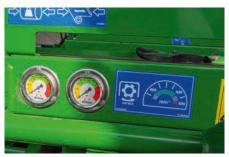
A choice of 540 or 1,000rpm input was offered from new, the latter allowing greater torque to be transmitted through the machine and so suiting chopping heavy material. The rpm decal indicates the most economical pto speed range. Two pressure gauges, for bale density and knife pressure, are not marked but in work both should be in the green area.
