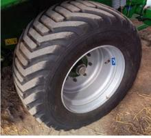
Standard tyres are 500/50-22.5 and are the most common fit. Wider 560/45-22.5 tyres are available, with non-chopper V640 or V6740 models having a slimmer 460/65-20 tyre as standard. An eight-stud axle was fitted from around 2014, but brakes remained an option although and 95% in UK will have hydraulic brakes. Air brakes are now an increasingly popular option.
