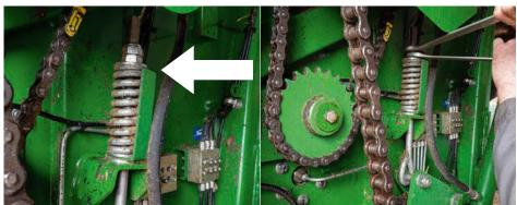
The roller drive chain tension is set by adjusting a spring, the correct setting seeing the top of the washer sitting level with the setting plate (arrowed). This is a simple setting to adjust (right) so be wary if a large adjustment is need as it could suggest a lack of service attention.
