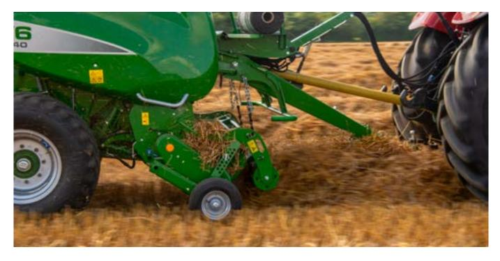
The new tapered feed channel encourages the crop to flow from the pick-up and then move towards the rotor and into the bale chamber, maximising throughput. McHale have also moved the lateral feed augers forward and their ends are angled towards the rotor for improved crop flow.
