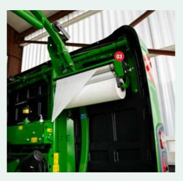
The dispensers are fitted with film break sensors, which notify the operator through the control console in the tractor cab if one or both dispensers run out of film. If one dispenser runs out of film the Fusion Vario Plus will continue working and automatically slow bale rotation and increase the number of rotations of the wrapping ring to ensure that the bale is wrapped correctly.
