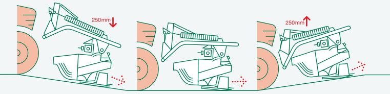
The Pro Glide front mower has its own independent suspension, which allows the mower to automatically move up & down independent of the tractor and has a vertical travel range of 500mm. If mowing into a dip, the angle of the cutter bar will automatically adjust down and while mowing into an incline the cutterbar angle will automatically adjust up.
